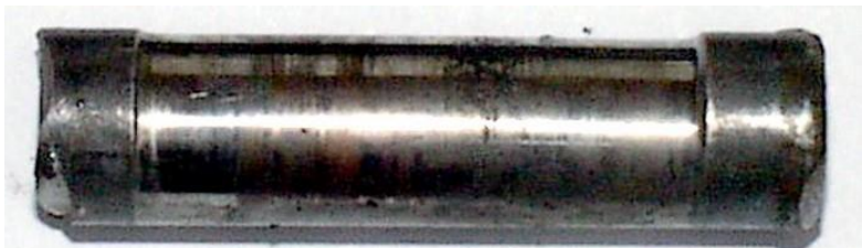
heavy wear on a roller chain pin
