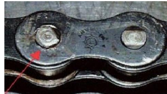
tilted pin caused by high friction forces
