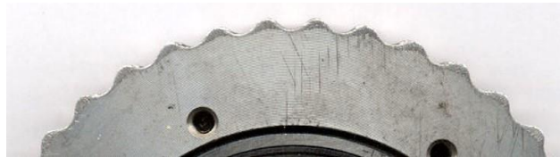
no maintenance (replacement) of sprockets
