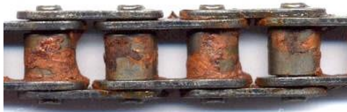
standard chain, lubricated, after salt spray test DIN 50021 SS
