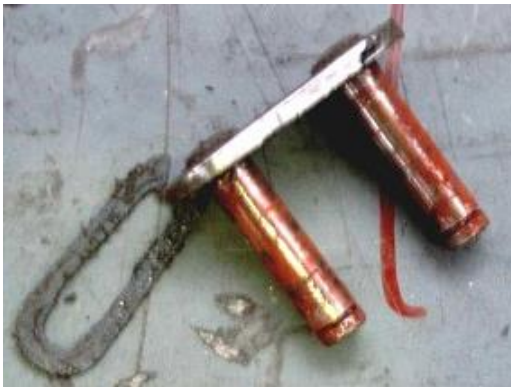
friction rust caused by dry run
