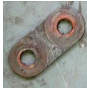
friction rust caused by dry run
